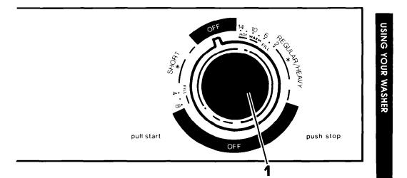
A warm wash is pre-set in the SHORT Cycle. Push in and turn the Control Knob so it points to the FILL bar. Pull the Control Knob out to start.
