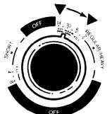
• When there is as much water as you want in the washer, push the Control Knob in. **SLOWLY** turn it to the right, past the fill area. Pull the Control Knob out.
