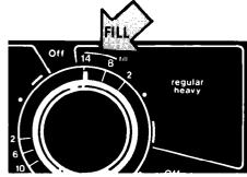
• The washer fills only when the Control Knob points to one of these "FILL" bars. For a lower water level, see page 5.
