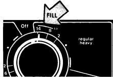
• To use less water, push the Control Knob in and turn to the right (clockwise) to a "FILL" bar in either the REGULAR HEAVY or SHORT Cycle. (PERMANENT PRESS fills to the highest level.)
