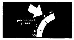
There is a dot just after the numbers in PERMANENT PRESS, REGULAR HEAVY and KNITS GENTLE. If you push in on the Cycle Control Knob, turn the pointer to one of those dots and pull the Control Knob out, the washer will fill, agitate, drain and spin. If you want high agitation and spin, use the dot in REGULAR HEAVY If you want low agitation and spin, use the dot in KNITS GENTLE. Use the dot in PER-MANENT PRESS if you want high agitation and a low-speed spin
