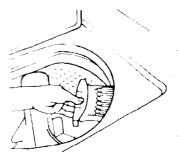
Water runs through the lint filter. whenever the washer agitates. Check it often to make sure its clean and filtering at its best
