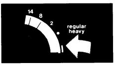
To set the washer so it drains and spins water out of the load, push in on the Control Knob, turn the dial to the right (clockwise) so the pointer is touching the bar just before OFF in any cycle. The washer will drain, spin out water and stop. If you want a low-speed spin, use the bar on PERMANENT PRESS or KNITS GENTLE All the other cycle settings have a high-speed spin. DETERGENT INFORMATION / DISPENSER / PRE WASH / RINSE ONLY / SPIN ONLY
