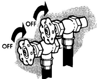
**WHEN NOT WASHING**, keep both water faucets turned off, this takes the pressure off the water inlet valve and hoses.
