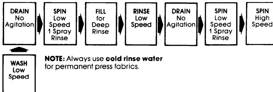
**\* IMPORTANT: THE WASHER WILL PAUSE BRIEFLY THROUGHOUT EACH CYCLE. These pauses are normal. They allow for the reversing of the motor, normal washer operation, and the cool down portion of the PERMANENT PRESS Cycle.**
