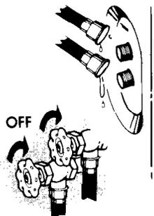
1. Shut off both water faucets. Disconnect and drain water inlet hoses.
