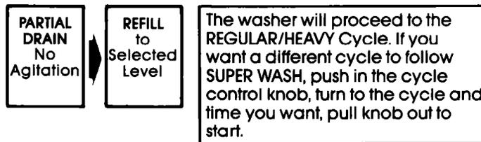
\* **IMPORTANT: THE WASHER WILL PAUSE BRIEFLY THROUGHOUT EACH CYCLE.** These pauses are normal. They allow for the reversing of the motor, normal washer operation, and the cool down portion of the PERMANENT PRESS Cycle.
