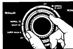
3. Set the washer for a DRAIN and SPIN (see page 12). Let it run for about 30 seconds to mix the antifreeze and water.
