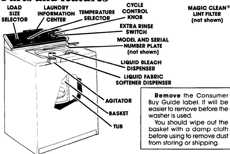
**Remove** the Consumer Buy Guide label. It will be easier to remove before the washer is used.
