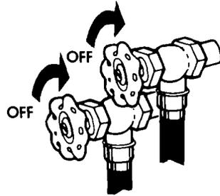
**WHEN NOT WASHING**, keep both water faucets turned off, this takes the pressure off the water inlet valve and hoses.
