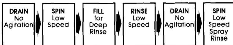
**NOTE:** THE WASHER WILL PAUSE BRIEFLY THROUGHOUT EACH CYCLE. These pauses are normal. They allow for the reversing of the motor, normal washer operation, and the cool-down portion of the PERMANENT PRESS Cycle.
