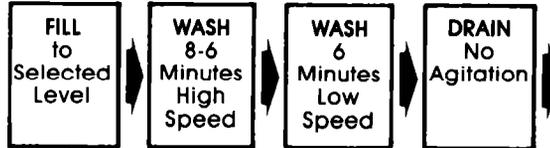
A cycle for sturdily constructed fabrics that are heavily soiled.
