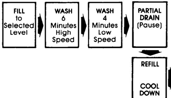
A cycle designed for moderately soiled permanent press and some synthetic fabrics. The **cool-down** rinse helps keep wrinkles from setting into these fabrics.
