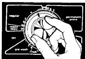
3. Set the washer for a DRAIN and SPIN (see page 10). Let it run for about 30 seconds to mix the antifreeze and water.
