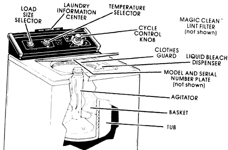
Remove the Consumer Buy Guide label. It will be easier to remove before the washer is used. You should wipe out the basket with a damp cloth before using to remove dust from storing or shipping.
