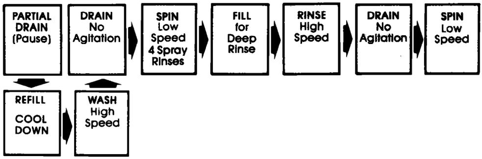
\* **IMPORTANT: THE WASHER WILL PAUSE BRIEFLY THROUGHOUT EACH CYCLE. These pauses are normal. They allow for the reversing of the motor, normal washer operations, and the cool down portion of the PERMANENT PRESS Cycle.**
