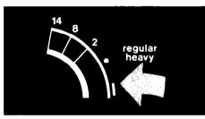
To set the washer so it drains and spiris water out of the load, push in on the Control Knob, turn the dial to the right (clockwise) so the pointer is touching the bar just before OFF in any cycle.
