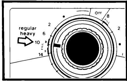
**WARM WATER** can be selected by turning the Control Knob to 8 or 10 minutes in the REGULAR HEAVY Cycle.
