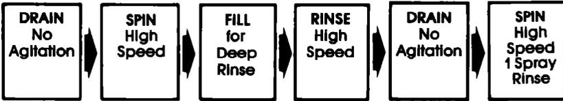
**\* IMPORTANT: THE WASHER WILL PAUSE BRIEFLY AT DIFFERENT TIMES IN EVERY CYCLE. These pauses are normal. They allow for the reversing of the motor and normal washer operations.**
