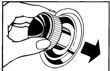
**D.** To stop the washer at any time push in the Control Knob. To restart the washer, pull out the Control Knob.
