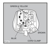
The wire coloured green and yellow must be connected to the terminal marked with the letter  $\langle E \rangle$  or by the earth symbol  $\perp$  or coloured green and yellow.
