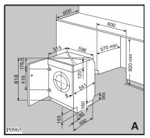
When installing the appliance into the kitchen furniture ensure, if possible, the hoses are placed in either of the two recesses on the back of the appliance. This will help to prevent the hoses from becoming kinked or trapped. Picture AB.
