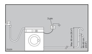
When discharging into a standpipe ensure that the top of the curve in the hose end is no more than 90cm (35.4") and no less than 60cm (23.6") above floor level. The upright standpipe should have a minimum length of 30cm (12") from the bottom of the elbow to the top of the pipe (see diagram).
