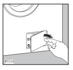
Place a container close to the pump to collect any spillage.  When no more water comes out, unscrew the pump cover and remove it. Always keep a cloth nearby to dry up spillage of water when removing the cover.
