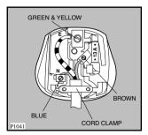
The wire coloured green and yellow must be connected to the terminal marked with the letter  $\ll E \gg$  or by the earth symbol  $\frac{1}{2}$  or coloured green and yellow.
