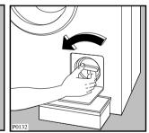
Unscrew and remove the filter.
