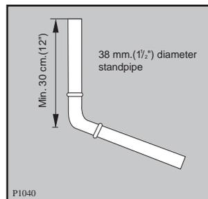
Make sure that it is designed in such a way, that the end of the drain hose cannot be covered with water.
