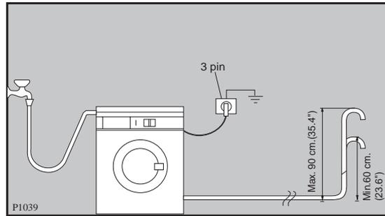
When discharging into a standpipe ensure that the top of the curve in the hose end is no more than 90cm (35.4") and no less than 60cm (23.6") above floor level. The upright standpipe should have a minimum length of 30cm (12") from the bottom of the elbow to the top of the pipe (see diagram).
