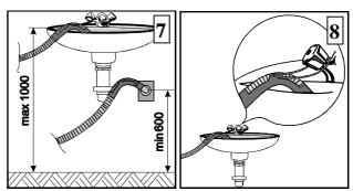
The end of the outlet hose should be raised from the floor by not more than 100 cm and not less than 60 cm. If the hose is positioned higher than recommended, the machine will not pump out the water.
