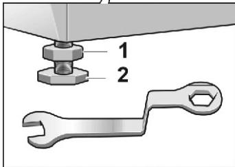
All four appliance feet must be firmly on the ground. The washing machine must not wobble
