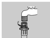
6. If the water tap is a screw type, assemble a water supply hose that fits to the tap as shown.
