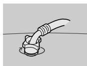
5. Connect the other end of the water supply hose to the inlet water valve at the top of the washer. Screw the hose clockwise all the way in.
