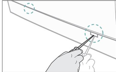
3. Unscrew the emergency drain cap by turning left. Grip the end of the emergency drain tube and slowly pull it out about 15 cm.
