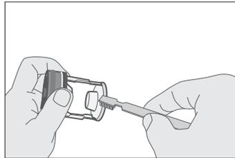
4. Wash any dirt or other material from the filter. Make sure the drain pump propeller behind the filter is not blocked. Replace the filter cap.
