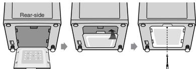
1. Insert the sound absorbing panel to the assembling hole on back side to the end
