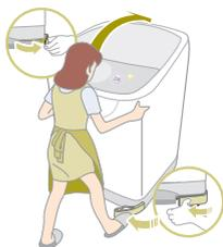
Pull the handles located at the right and left of the front side and slide off.
