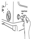
Be sure to join tightly the drain hose into the drain-outlet on the back of the machine.
