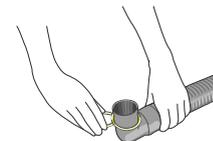
2. After directing the drain hose to a drain, join to the drain-outlet of the washing machine.
