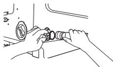
Install the drain hose in the position of about 90~100cm above the ground.
