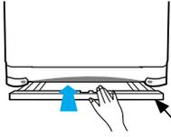
2. If you have difficulty inserting the panel lift up the washer a little and insert it
