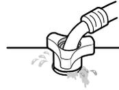
3. Check if there is a leakage. Note to tighten up the connector.
