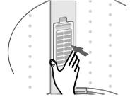
4. Close the cover and insert the lower part of the filter in the basket first and then push the filter with "click" sound.
