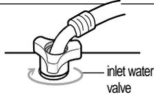
2. Pull in the filter and connect the hose to the inlet water valve tightly.
