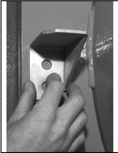
Figure 1: Mounting Accelerometer, 36030F8
