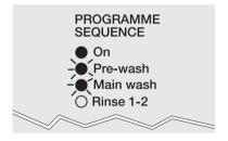
The "ON" lamp will illuminate and the "Prewash" and "Main wash" lamps will flash.
