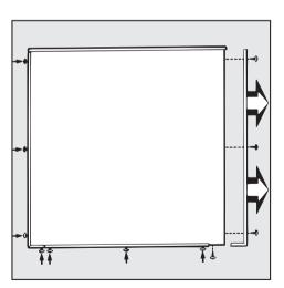
Remove the 4 screws from the decor strip on the door catch side of the door and remove the decor strip. ■ Unscrew the remaining 7 screws from lower and side decor strips until the decor panel bows slightly and can then be taken out or put in place.
