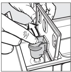
■ Remove the siphon tube from compartment <sup>®</sup> and rinse in warm water.
