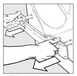
■ Withdraw the two struts together with the support plate.
