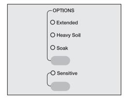
Select the desired "OPTIONS". Press the upper button until the indicator of the desired wash option lights.
