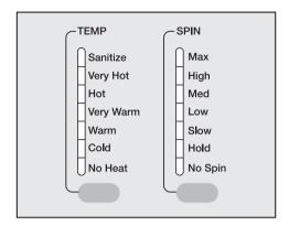
■ Press the "TEMP" and "SPIN" button until the indicator of the desired value lights.
