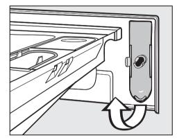
To clean the lint trap, remove the tool from behind the detergent dispenser drawer.
