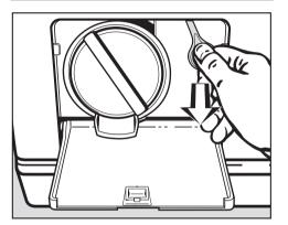
To open the door, pull down on the ring in the upper right corner of the access area.
