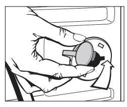
Close the holes with the rotary protectors, making sure to close the caps.
