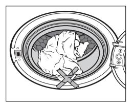
To prevent damage to the door seal and clothing, make sure that there are no clothes caught between the drum door and the seal.
