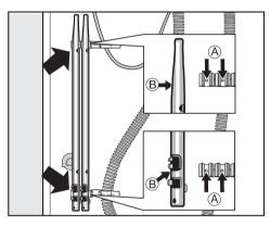
Fasten the shipping struts to the rear of the washer. Take care to insert the drill holes correctly, (B), into the clamps, (A).
