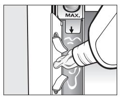
Add the fabric softener, mild liquid starch or starch to compartment %.
