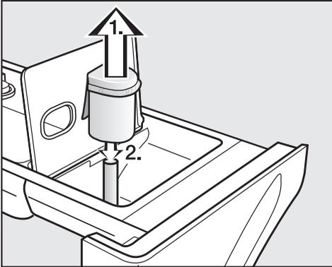
1. Remove the siphon tube from the "Softener" compartment and rinse under warm water. Also clean the pipe connected to the siphon tube.
