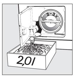
■ Turn the lint trap lid counterclockwise 2-3 times. Do **not** remove it. Approx. 2 litres (2 quarts) of water will drain out of the hose.
