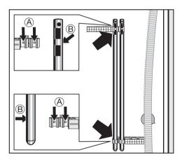
■ Fasten the shipping struts at the rear side of the washer. Take care to insert the drill holes (B) onto the spigot (A).
