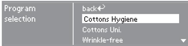
All pre-set programs can be selected with the jog shuttle. Depending on the direction the jog shuttle is turned the highlighter moves up or down. The arrows ▼▲ at the right side of the display show that more selections are available. Press the jog shuttle to open the basic menu of the selected wash program.
