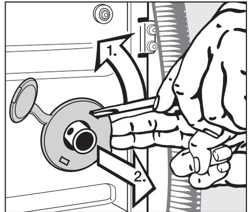
1. Unhook the rotary protector with a screw driver.
