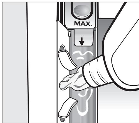
The softener or liquid starch is automatically dispensed in the final rinse. At the end of the program a small amount of water remains in the fabric softener compartment ☼.
