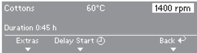
The program components (program, temperature and spin speed) can be selected by turning the jog shuttle. The selected component is highlighted. Press the jog shuttle to select the component. The respective submenu is displayed.
