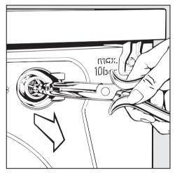
Using needle nose pliers, withdraw the plastic filter by pulling on the bar (see illustration). Rinse under water to clean, and then replace.
