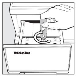
Turn the dial to the desired setting. Use the tool supplied with the machine. It is located behind the detergent drawer, on the left hand side (see Cleaning and Care) water.
