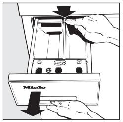
Press down the red release lever and, at the same time, pull the drawer out of the machine.
