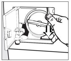
Pull down the ring in the upper right corner of the access area, and the door will open.
