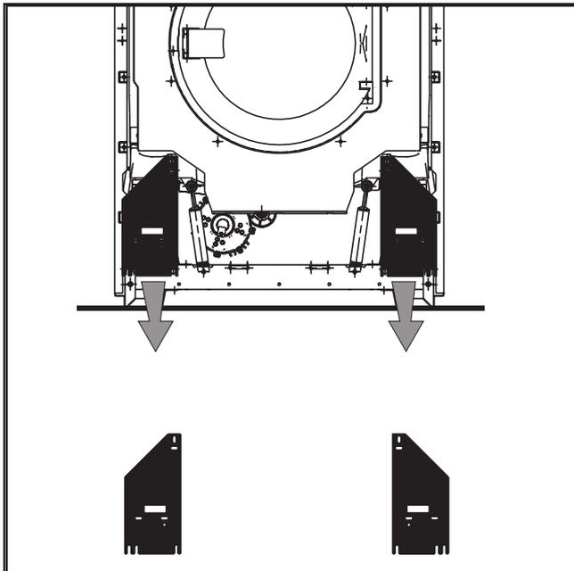
Four red-marked shipping struts, two at the front and two at the rear, are each fixed with 3 hex screws.
