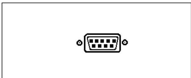
A serial interface is located at the rear of the washer to connect the machine to a PC (Personal Computer).
