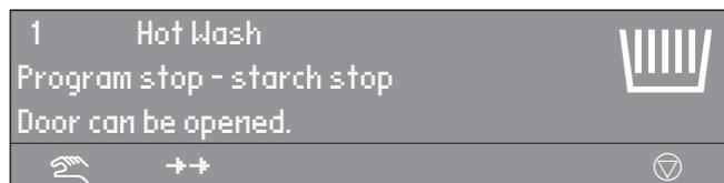
"Program stop - Starch Stop" flashes in the display when it is time to add starch to the laundry.
