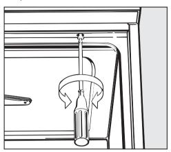
■ Secure the machine to the front edge of the worktop using screws through the holes on the left and right hand sides of the front trim.
