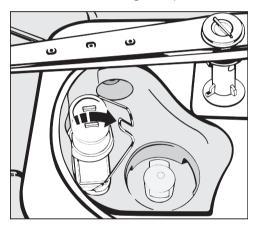
■ Lift up the non-return valve and rinse under running water.
