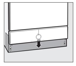
■ Pull the emergency release cable (located at the bottom of the machine behind the service panel) downwards to open the door.
