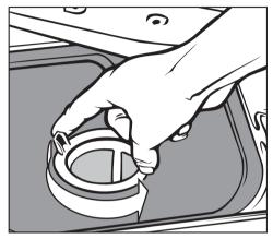
■ To unscrew the micro-fine filter, grasp the two tabs and turn counterclockwise twice.
