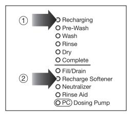
When the salt reservoir is empty the "Recharge Softener" indicator, ②, illuminates to remind you to fill the reservoir.
