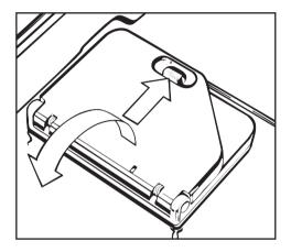
Press the opening catch on the container forward. The flap will spring open. The flap is always open at the end of a program.
