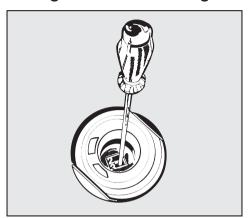
The dosage adjuster (see arrow in the illustration) in the opening has settings adjustable from 1 to 6 (1 - 6 ml). It is preset to "3" (3 ml).
