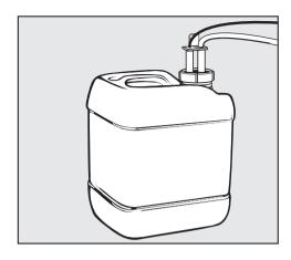
■ Insert the siphon tube into the container (observe the color code).
