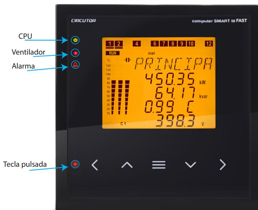
Figura 15:Indicadores LED del Computer SMART III FAST.
