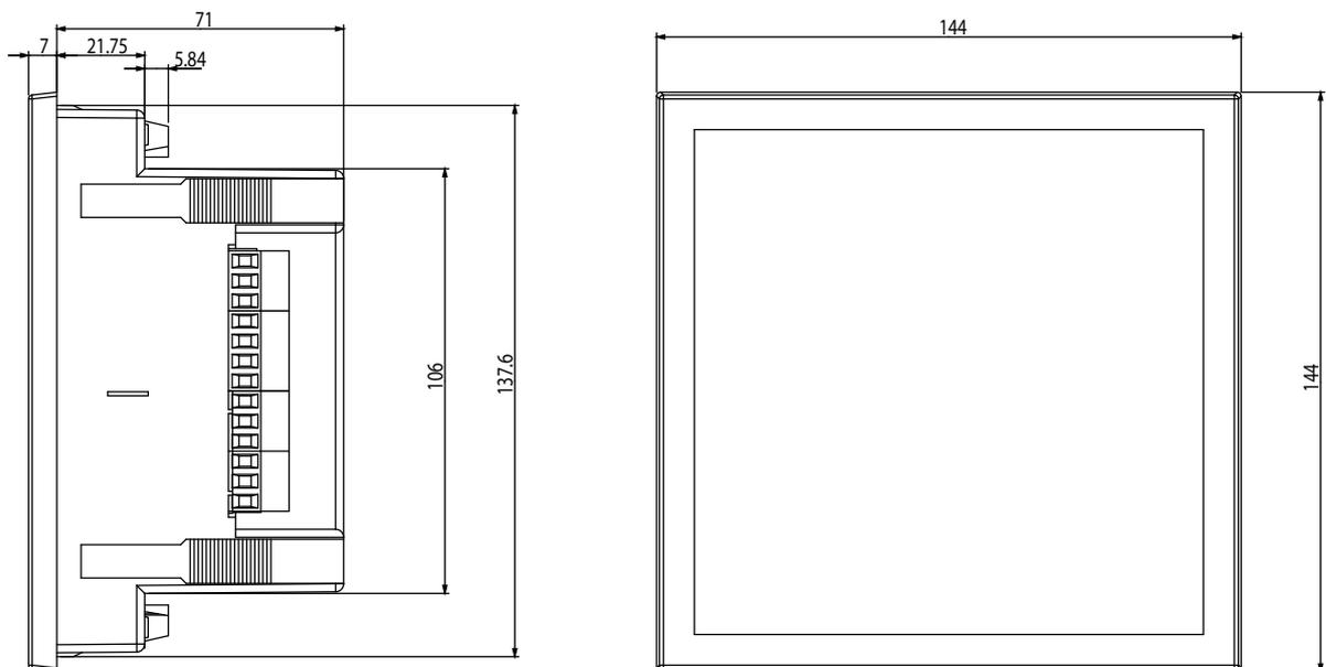
Figura 19: Dimensiones del Computer SMART III FAST.
