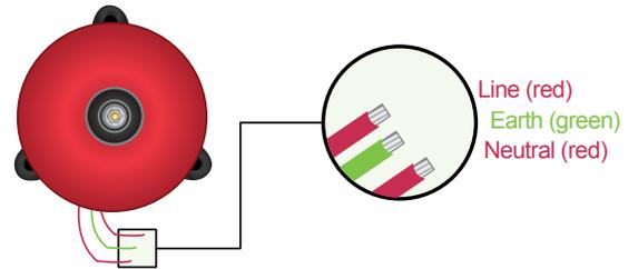
4. Connect the bell in accordance with the connections diagram.
