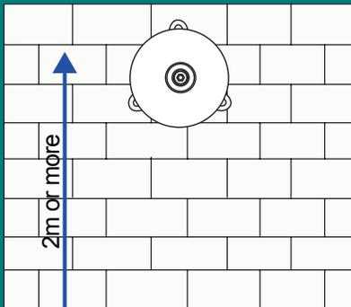
2. Take as reference the bell base, mark and drill holes. Then insert wooden pegs.
