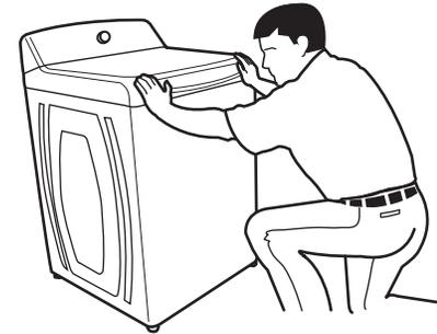
3. Lower right front foot until it contacts the floor. By hand, firmly rotate foot as much as an additional 1½ turns. The other three feet have been preset at the factory.
