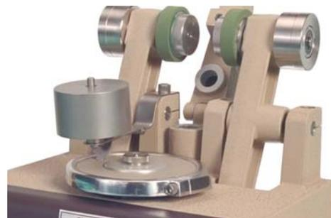
Used in place of the abrasive wheels, the Scuffing Head Attachment is mounted on the inside riser mount for the left abramer arm. The abramer is operated in the normal fashion, however the vacuum system is not utilized. With a hinged design, the scuffing tool may be raised when not in use.
