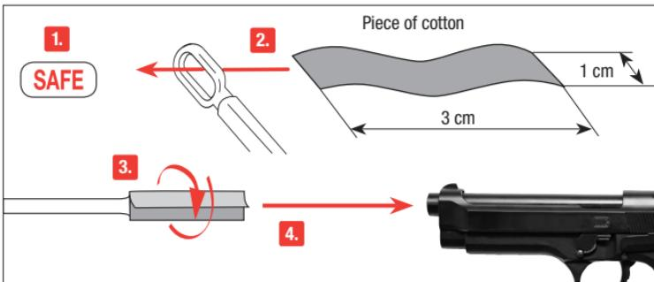
Put the safety on "safe". Prepare a thin rod with a length of approx. 30 cm. Attach a piece of cotton fabric to its end and clean the barrel with some silicone oil.
