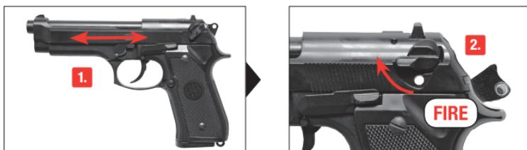
To cock the pistol pull the slide to the end and push the slide back to front position
