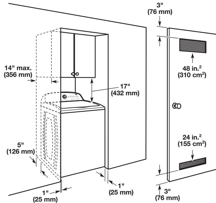
Select proper location for your washer to improve performance and minimize noise and possible "washer walk". Install your washer in a basement, laundry room, closet, or recessed area.
