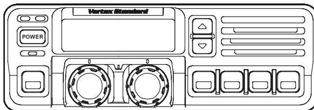
The VX-6000 Series are full-featured FM transceivers designed for flexible mobile and base station business communications in the VHF Low-Band (120/50 Watts: programmable), VHF High-Band (110/50 Watts: programmable) and UHF (100/50 Watts: programmable) Land Mobile Bands. Each model is designed for reliable business communications in a wide variety of applications, with a wide range of operating capability provided by its leading-edge design.
