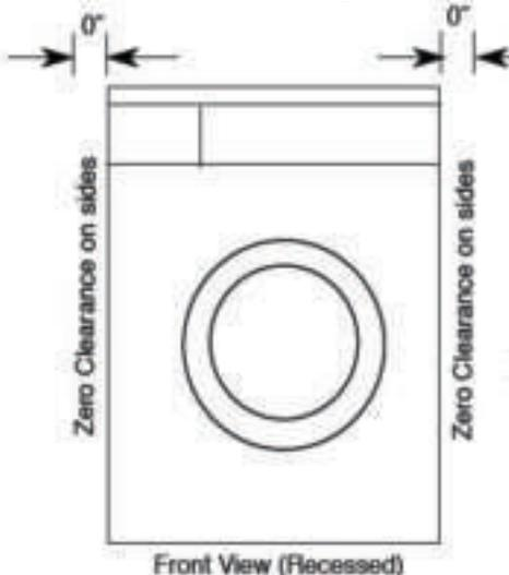
If the appliance is to be installed in a closet, the installation must be completed by a qualified person or service representative. Adequate blocking to secure unit is required. Additional clearances for floor, wall or door moldings may be required.
