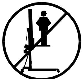
**3.1** - The TL-070 is a machine designed to elevate loads upwards in a vertical direction, NEVER should it be used as a platform to elevate people.
