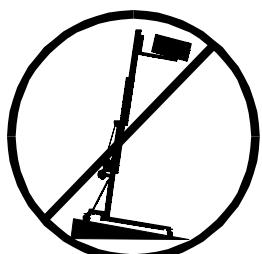
**3.2** - Only place the lift on hard, flat surfaces always checking that it is in a vertical position by using the bubble level indicator (**F**) found on the base section. Adjust the outrigger stabilisers (**Q**) by turning the cranks to level if necessary. NEVER use wedges or other foreign objects to bring the lift to equilibrium.
