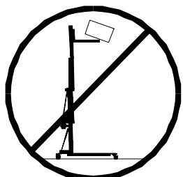
**3.4** - NEVER should the lift be used to elevate a load that has not been properly checked. It is necessary to verify that the load is correctly supported and centred on the appropriate lift support so that the weight of the load will only elevate in a vertical direction.
