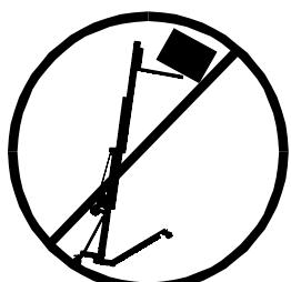
**3.3** - Check that the outriggers are placed and set-up correctly using the pins safety system.
