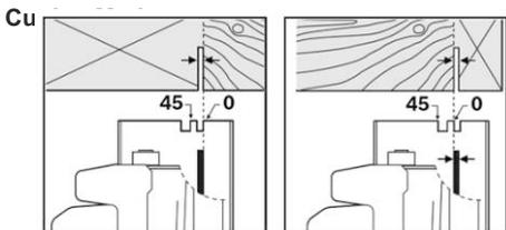
The 0° cutting mark (10) indicates the position of the saw blade for right-angled cuts. The 45° cutting mark (9) indicates the position of the saw blade for 45° cuts.
