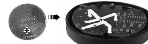
The battery has to be changed if the symbol appears in the display during the measurement. Open the housing using a screwdriver. Remove the used button cell. Put in new button cell - **Observe polarisation!**
