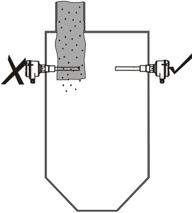
**Caution:** Protect shaft and tines from falling material.
