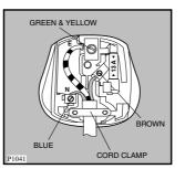
The wire coloured green and yellow must be connected to the terminal marked with the letter «E» or by the earth symbol  $\perp$  or coloured green and vellow.
