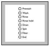
The "**End**" pilot light flashes in the event of operating problems. And the relative alarm code appears on the display.
