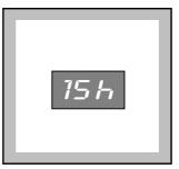
The delay time is displayed for 3 seconds, then the duration of the selected programme reappears. After you have pressed the Start/Pause button, the countdown begins, and the delay time value decreases by one unit every hour up to 2 hours and then by 30 minutes.
