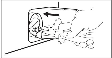
8. Remove foreign bodies and fluff from the pump seat and from the pump impeller.
