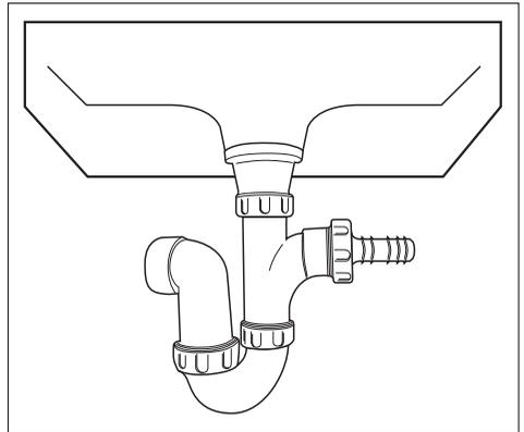
Push the drain hose onto the spigot and secure with a clip, ensure a loop is formed in the drain hose (see diagram) to prevent waste from the sink entering the appliance. If you intend to drain the hose from the machine into a sink, make sure that the sink is empty and the plug hole is not blocked. Use the plastic “U - Piece” supplied.
