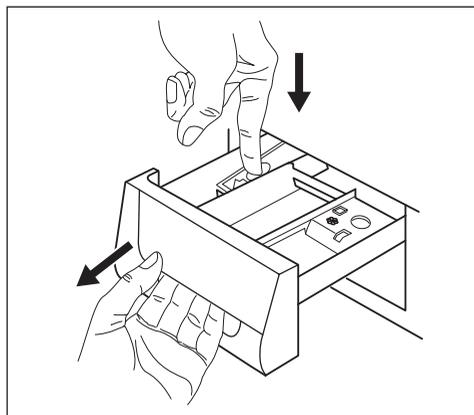
To aid cleaning, the top part of the additive compartment should be removed.
