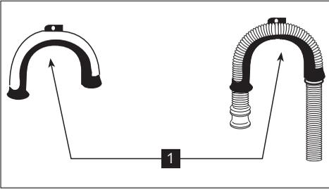
Place the drain hose into your standpipe, which should have an internal diameter of approximately 38 mm thus ensuring there is an air break between the drain hose and standpipe.
