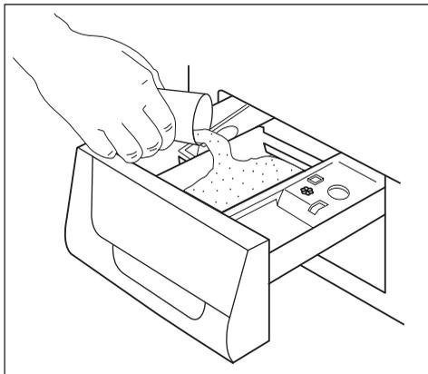
If required, pour fabric softener into the compartment marked
