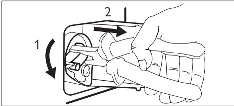
11. Replace the emergency emptying cap into the filter cover and fix it firmly.
