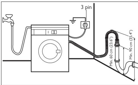
The drain hose may be extended to a maximum of 4 metres. An additional drain hose and joining piece is available from your
