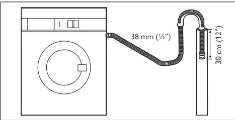
When discharging into a standpipe ensure that the top of the standpipe is no more than 90 cm (35.4") and no less than 60 cm (23.6") above floor level.
