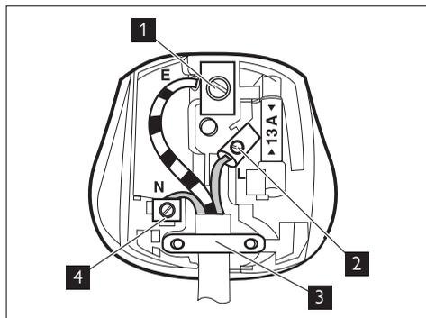
The wire coloured green and yellow must be connected to the terminal marked with the letter «E» or by the earth symbol  $\perp$  or coloured green and yellow.
