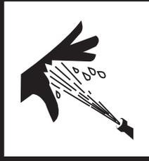
Water under pressure may cause serious injury. Do not point spray nozzle at any part of the body or place in mouth. Do not point spray nozzle at any persons.
